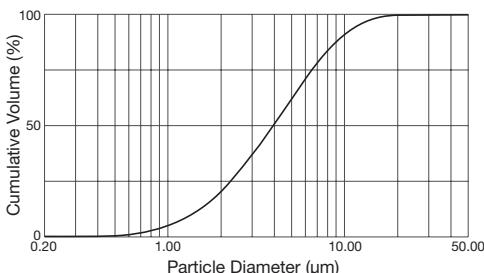
All measurements were obtained with a sodium chloride solution using a laser diffraction method.
